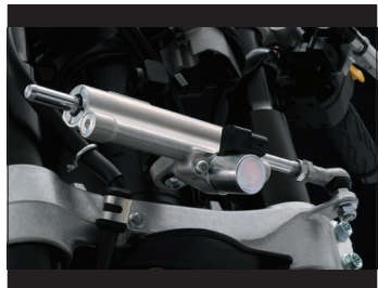
Electronically controlled steering damper
